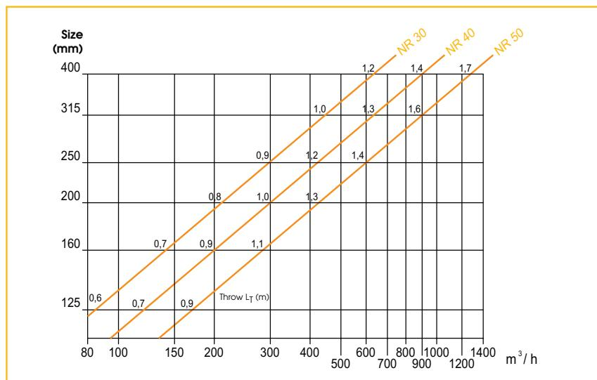
Throw factor is based on a  $v_R$  of 0,17 m/s in the occupied zone.
