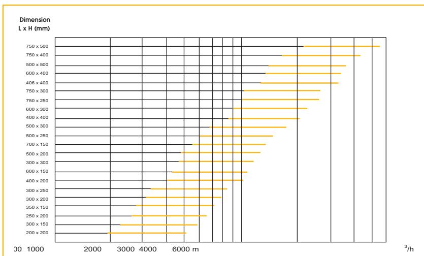
The selection area is based on a  $v_f$  between 2 and 5m/s.
