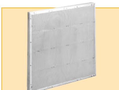
**Activated carbon filters mod. CAP** are flat panels made of a supporting steel sheet frame superficially protected by electrolytic galvanization and micro-drawn grids. The activated carbons are positioned inside; there are also anti-sagging rigid elements.
