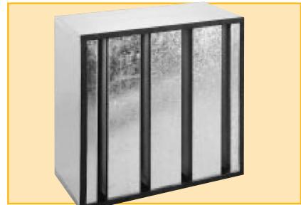
Prodotto: **SAF**Maximum air flow rate: **160 % of nominal**Maximum operating temperature: **60 °C**Maximum relative humidity: **60 %**Applications: odors, steam and organic solvents: **Carbon type 2.0**Application: acid gas, H<sub>2</sub>S, SO<sub>2</sub> etc.: **Carbon type 2.1**Application: formaldehyde: **Carbon type 2.2**Application: nuclear, radioactive isotope, radioactive nuclide: **Carbon type 3.0**Optional: construction: **AISI 304 stainless steel**
