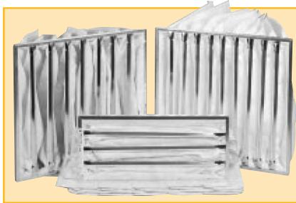
The range of Filtra-Pak V bag filters covers a very wide performance range and meets the requirements of numerous civil and industrial facilities. These filters have medium and high efficiency rates, with limited pressure drops. This means fan energy consumption is limited. The filter media are made of glass fiber, self-extinguishing non-woven textile, progressively structured, coupled with a support sheet on the air outlet side that reinforces and protects the structure.
